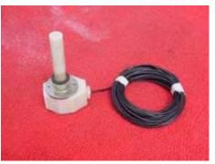
Ag/AgCl Reference Electrode we designed consists of two kinds: Permanent Ag/AgCl Reference Electrode and Portable Ag/AgCl Reference Electrode. We also could design the products according to customers' requests.
