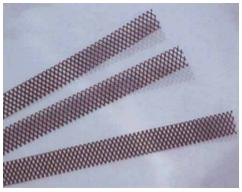
the catalyst is Mixed Metal Oxide. Titanium expanded grid substrate coated with lrO<sub>2</sub>/Ta<sub>2</sub>O<sub>5</sub> and meet ASTM standard B265 grade 1 or grade 2.
